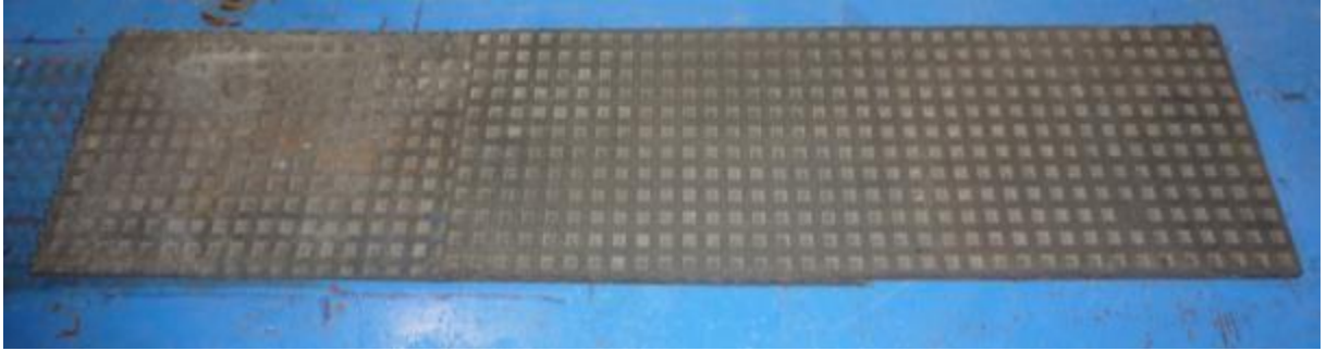
Figure 22: Neoprene pads used to simulate support conditions
